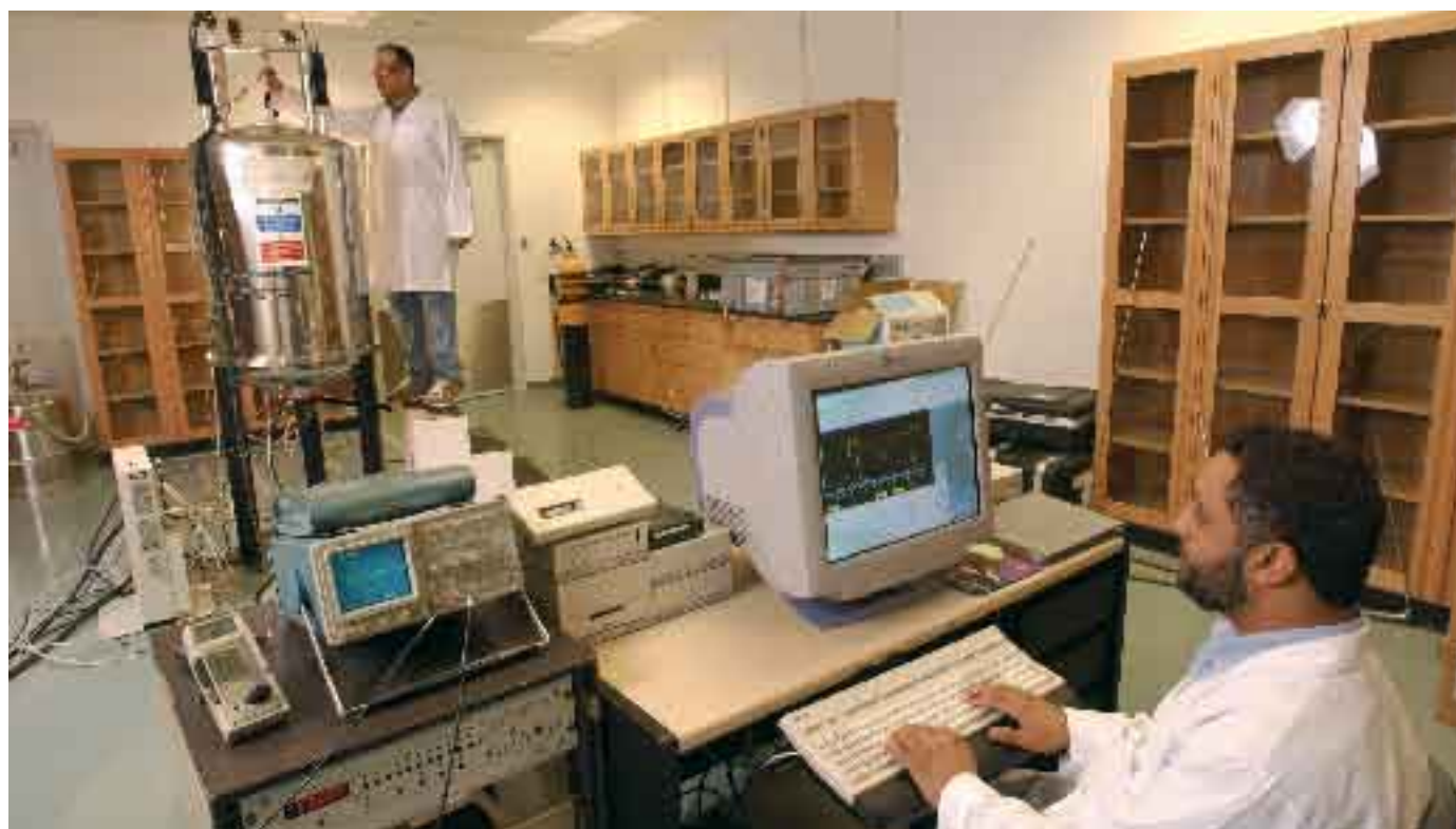
Lab technician specialist Abdulrahman Al-Nowaishi (at computer) and lab technician Marwan Al-Dossary perform a Nuclear Magnetic Resonance (NMR) analysis.
