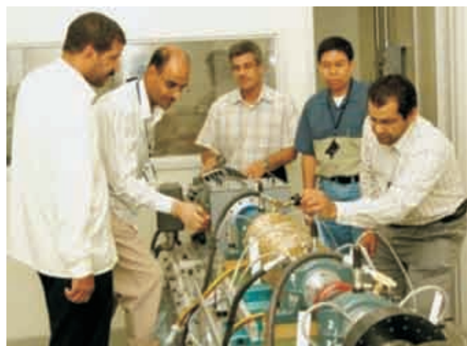
Dynamic Analysis Unit members Yousif Al-Sahood (on short-term assignment), Fathi Al-Salem, Khaleel Al-Hussain, Joveth Abutas and Ghaib Al-Motairi examine the Rotordynamic Test System at the Research and Development Center in Dhahran. The equipment was tailor-made for Saudi Aramco and designed by Spectraquest Inc. with substantial input from the Consulting Services Department. It is the only one of its kind in the Middle East. (Photos by Abu Abdul Aziz Studio)
