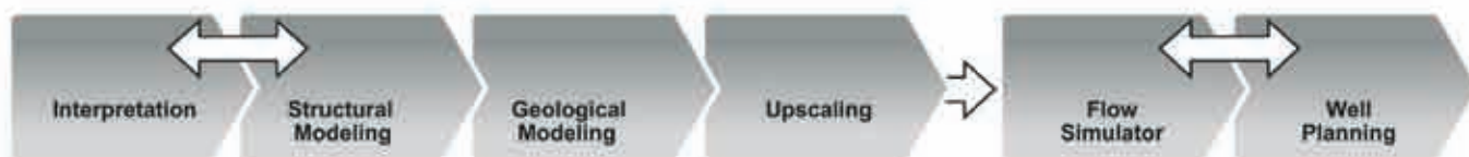
Figure 1 - Linear Workflow commonly used to generate reservoir models.
