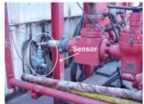
Fig 4. Assembly of the pressure sensor at the choke manifold.
