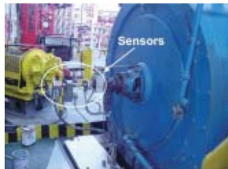
Fig 1. Assembly of the hook height sensor at the drawworks
