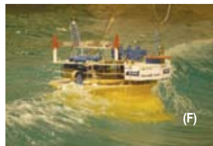
(a) (b) and (c) Details of the MONOBR model; (d) MONOBR model in still water with all mooring and riser lines; (e) and (f) MONOBR in hurricane condition with waves of significant height of 17.50 meters and peak period of 16.3 seconds and current of 1.4 m/s associated with wind of 60 m/s.
