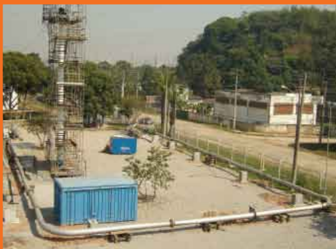
14" diameter loop - 120 meters in length.
