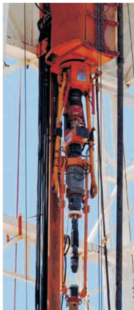
Figure 3: Top Drive and Casing Drive Assembly (from Tesco website)
