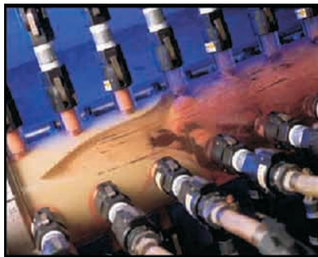
Figure 5 - Detail of the Gravel Pack Simulator
