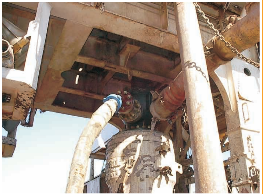
Figure 2 – Rotating head and the connections to the manifold. Drilling procedures, including tripping and connections were all normal, without changes.
