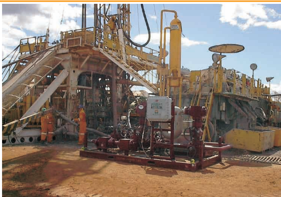
Figure 1 – Manifold in use during the first well for Petrobras in Brazil. The small footprint was an important factor in gaining the rig crew's acceptance.
