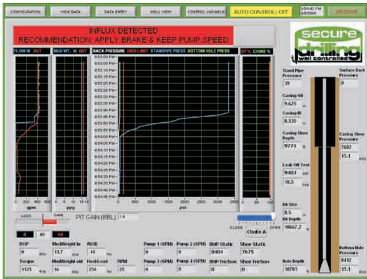
Figure 6 – Influx detected during one connection. Observe the difference from the normal behavior shown above.
