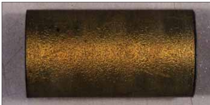
24-carat gold film prevents gas leaking from the core under hydrothermal conditions.
