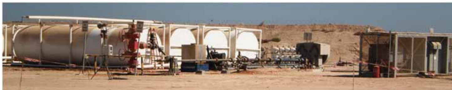
Figure 4: The use of modular equipment facilitated transportation and setup in the desert and added flexibility to the system design as items were substituted to improve reliability. [SOURCE: OTC 21130 Figure 2]
