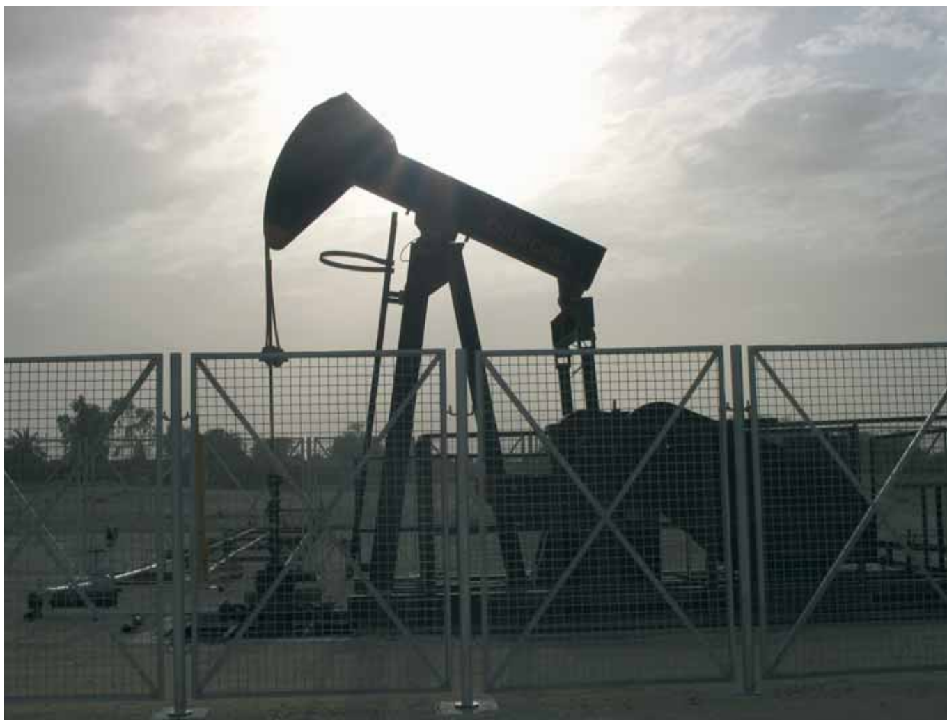
Figure 1 - Nodding Donkey Or Rod Pump (EPRasheed)
