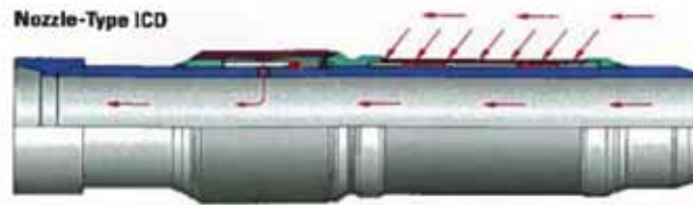
Figure 1: Typical Nozzle Based ICD with wire wrapped screen
