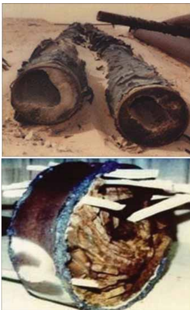
Fig. 1. Severity of \text{CaCO}_3 scaling in the Ghawar field before scale inhibitor treatments.
