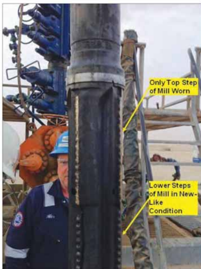
Fig. 6. Picture of step mill after retrieval back to surface.
