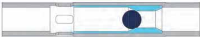
Fig. 2. Ball-activated port showing ball seat of a multistage fracturing completion: Open/Final position.
