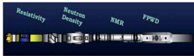
Fig. 5. LWD tool string used for horizontal injector well placement.
