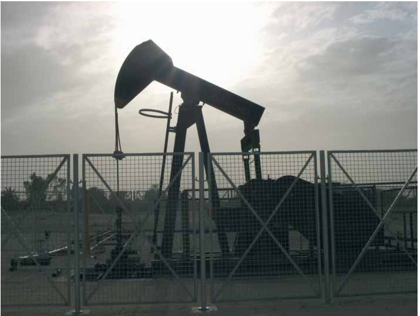
Figure 1 - Nodding Donkey Or Rod Pump (EPRasheed)
