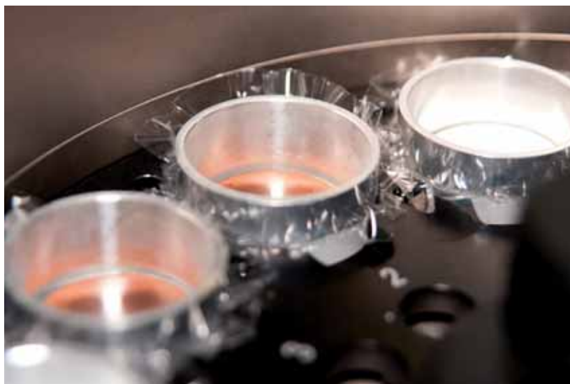
Figure 5: X-ray fluorescence (XRF) instrument is used to perform whole-rock elemental analyses at wellsite. Photo shows sample pellets ready for measurement in the XRF.
