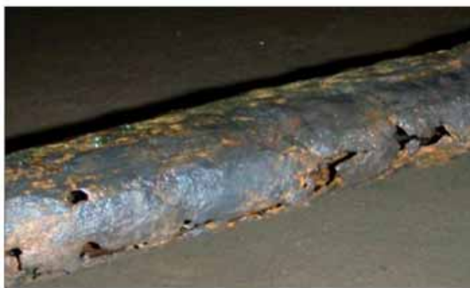
Fig. 1. Corroded tubing pulled out from one of the wells in the subject field.
