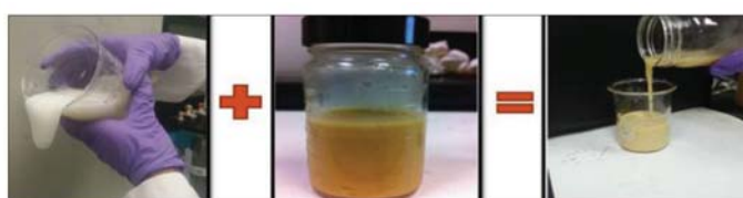
Fig. 5. Crosslinker stability test when mixed with emulsified acid and no internal breaker.
