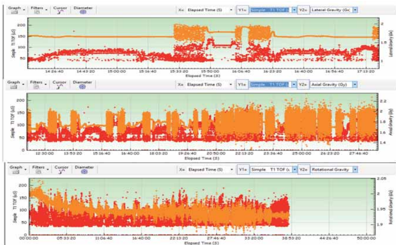
Fig. 9 plots Time and Vibration (Rotational, Lateral and Axial) and Time of Flight (TOF) measurements.
