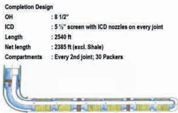
Figure 4 - Sandstone ICD completion with packers for every second joint.
