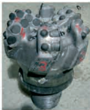
The photographs show the 8 1/2" DSX184M that reached TD in Well-B. The chamfered RazorEdge feature can clearly be seen on the cutters which remain in very good condition. The rig grading for this bit was 1-1-CT-A-X-I-TD.
