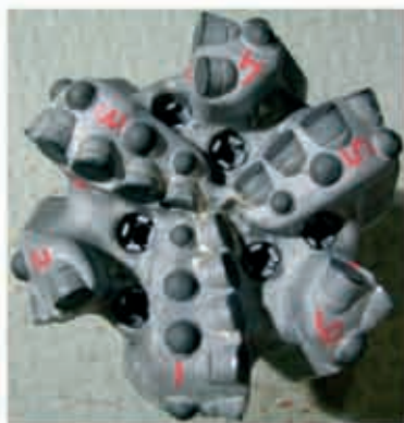
The photographs show the 8 1/2" DSX184M that reached TD in Well-B. The chamfered RazorEdge feature can clearly be seen on the cutters which remain in very good condition. The rig grading for this bit was 1-1-CT-A-X-I-TD.
