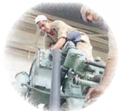
Saudi employees preparing gm/v-12 marine engine for dynamometer test. Dhahran, November 1968. Photo by: S. M. Amin
