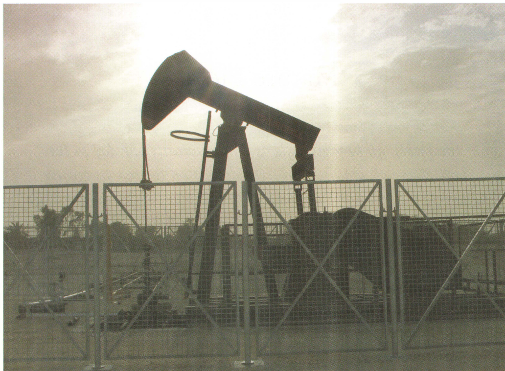
Figure 1 - Nodding Donkey Or Rod Pump (EPRasheed)
